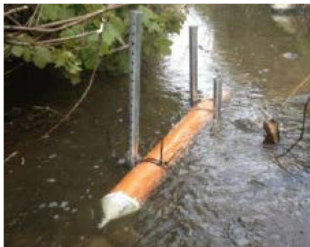
Figure 1: A time-integrated suspended sediment sampler deployed in Arable B.
