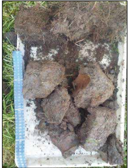
Figure 2 B. A sample exhibiting poor structural quality
