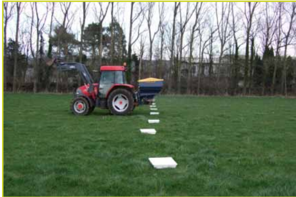
Figure 2. Determining the evenness of fertiliser spreading by Tray Testing
