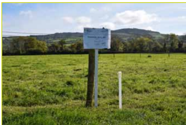
Figure 1 A Piezometer is installed to 4.5m depth to enable groundwater samples to be tested. Also such pipes allow us to examine the speed and direction of groundwater flow.
