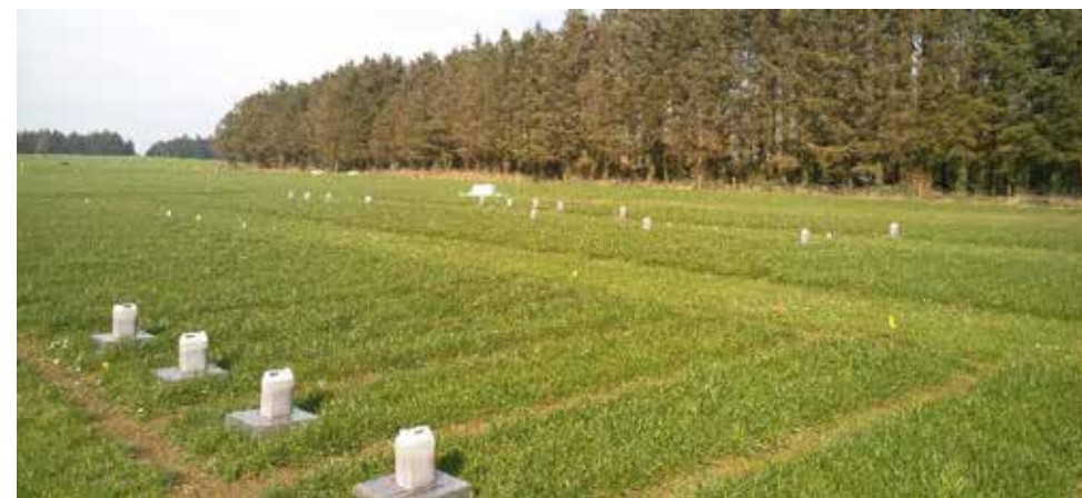
Figure 2. Measurement of greenhouse gas emissions with the installed chambers
