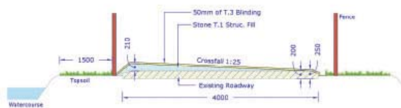
Figure 1- Farm Roadway resurfaced with T.1 Struc. fill and dust to a 1:25 crossfall away from stream
