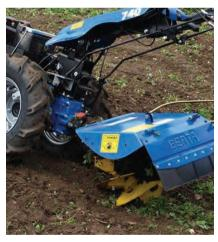
Two-wheel tractor and rotary plough in action.
