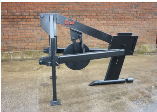
Figure 12. Mole plough showing cylindrical foot and expander
