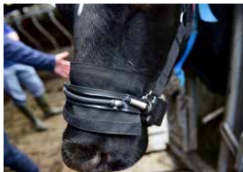
Figure 1. Protective casing of ITIN+HOCH Rumiwatch noseband sensor opened
