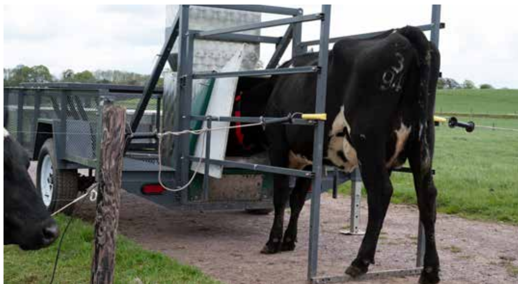
Figure 1. GreenFeed machine used to measure methane emissions in a pasture based system
