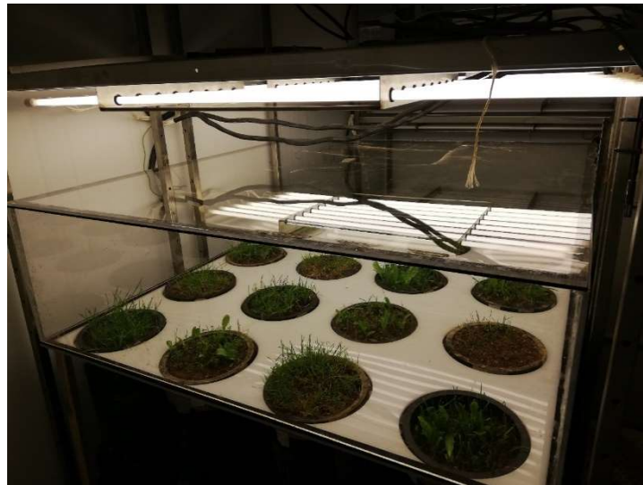
Fig. 4 Completed chamber construction with the engraved 10 mm opaque acrylic laid horizontally over the lysimeters with the 8 mm acrylic side panels and roof.
