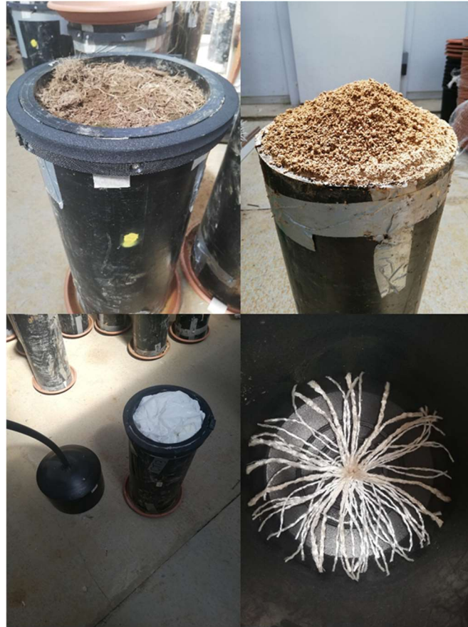
Fig. 2 Various stages of the lysimeter setup: gasket with neoprene lining (top left), inverted lysimeter with 4 mm sieved soil (top right), end-cap + hydrodare pipe with lysimeter prior to inversion (lower left) and the braided fire rope fanned out within the end cap (lower right).
