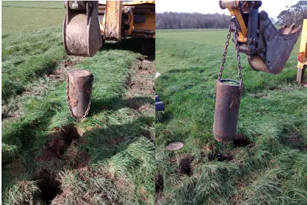
Fig. 1 The lysimeter extraction process before (left) and after (right). Lysimeters were housed in the cast iron shoe and drilled into the soil, before being retrieved with the JCB digger (see description above).
