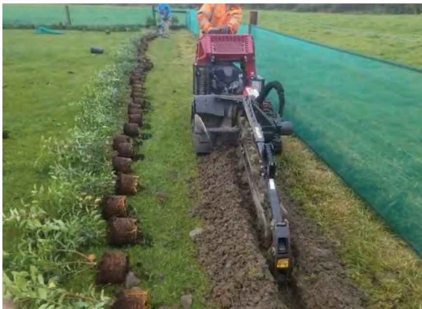
A trencher positioned 1.2m away from boundary fencing planting 3 Lt potted prunus with a wind-breaker attached to the boundary fence.
