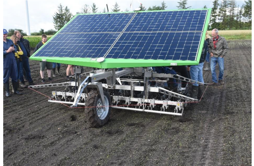
Farmdroid FD 20 with solar panel
