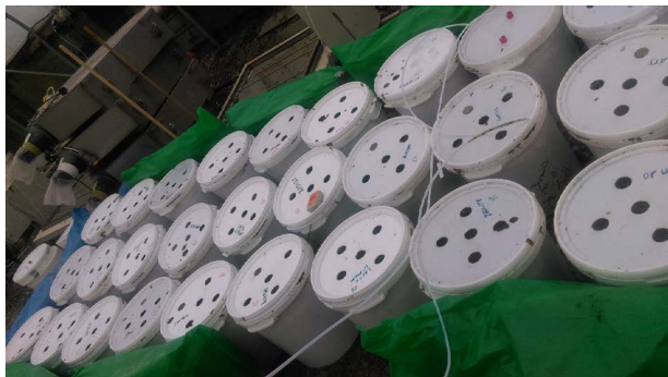
Figure 1. Medium scale slurry storage experiment in which multiple slurry amendments were examined
