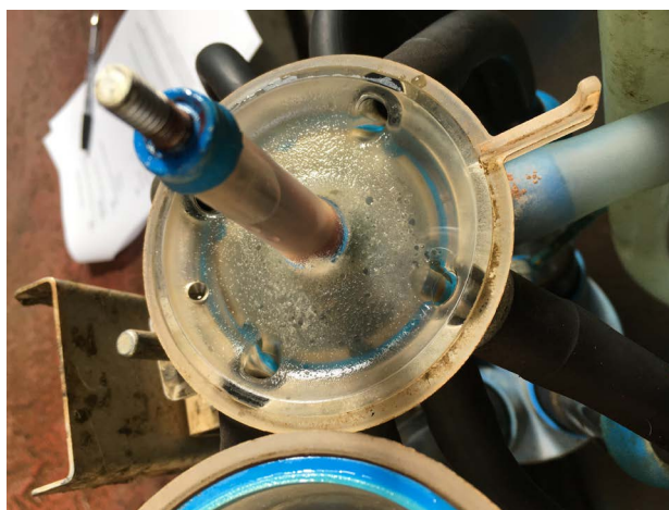
Figure 1. Residue build-up on a claw bowl
