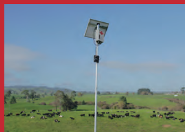
...Solar router retrieving live cow data from the field.
